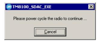
To continue, <u>remove</u> the DC supply to the radio and wait 5 seconds then re-apply DC supply
